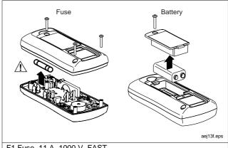
F1 Fuse 11 A, 1000 V, FAST. Minimum Interrupt Rating 17000 A.
